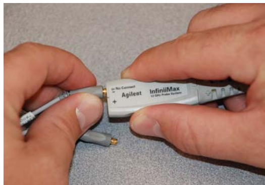
Figure 11 Properly Pulling the Probe Head Straight Out
