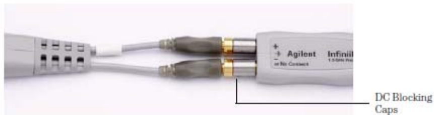
Figure 9 Placement of DC Blocking Caps Between Probe Amplifier and Head
